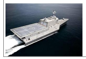
And then there's the massive helo' deck, big enough for a CH-53. This was the LCS they wanted because of the huge storage capacity under that flight deck and the size of the flight deck. Note that there is very little spreading wake. In fact, it does not look like a wake at all, just foamy water from the water jets. Somehow, at 43 knots, you'd think there'd be more of a wake.
