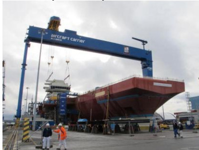
The 700-tonne navigation bridge of HMS Queen Elizabeth is lowered into place at Rosyth shipyard in Scotland
