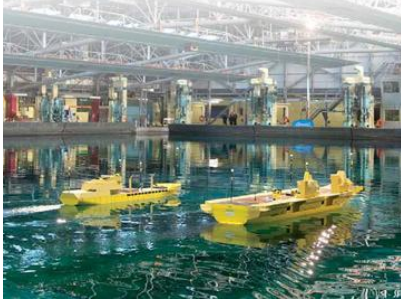
Close formation experiments with 1:44 scale models in the manoeuvring basin at Haslar
