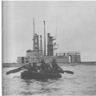
Perch (ASSP-313), during exercises with reconnaissance troops from the 1st Marine Division off the coast of California. In addition to many internal changes, the Perch's conning tower structure had been extended and additional masts and shears added by January 1957, when this photo was taken. USN photo and text from The American Submarine by Norman Polmar, courtesy of Robert Hurst via Navsource
