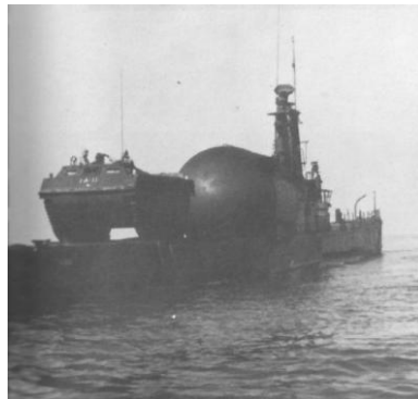
Yes, this IS a submarine with an Amtrak aboard. Perch (ASSP-313) preparing to launch an LVT amphibious tractor during a 1949 exercise. The vehicle could be carried in the cargo hangar and launched by flooding down the submarine. USN photo and text from The American Submarine by Norman Polmar, courtesy of Robert Hurst.
