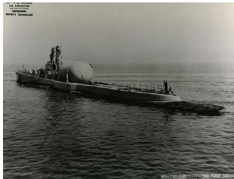
Aft view of the Perch (SS-313) off Mare Island after completion of her conversion to a troop transport. Note the large dry deck shelter for equipment and small boats. US Navy photo
