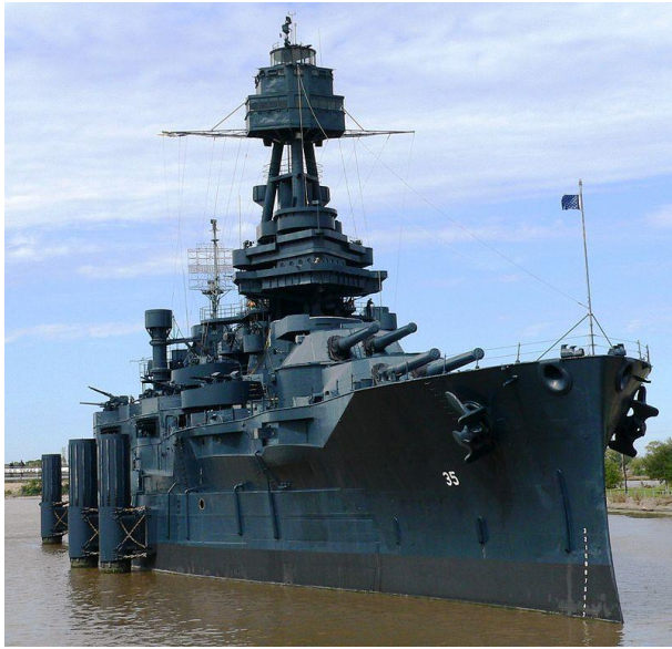
USS Texas in San Jacinto State Park, October 2006. The battleship is painted as it was in 1945 with Measure 21, Navy Blue System Camouflage. The camouflage was intended to make the battleship more difficult to detect from the air.
